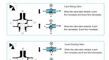
\*Remark: DN40~DN65 3-port valve only has mixing valve, if diverting is needed, just exchange port A and AB and follow the plate instruction.
