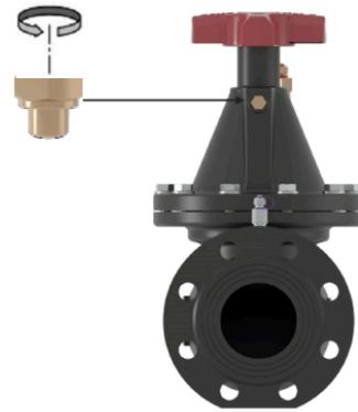
3. Use the hydraulic debugging instrument to measure the DP between P2 and P3, insert the measuring probe into the test plugs of the DPCV, rotate the handwheel, observe the DP on the instrument, and adjust the set DP; When  $\Delta H > 2 * \Delta P_{set}$ , DPCV starts to work.
