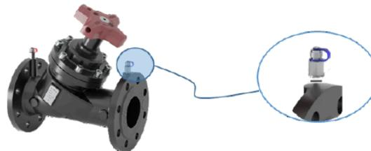
3. Open the 3-port test plug of DPCV and screw it into the low pressure end of the static balancing valve. After the 3-port test plug is installed, tighten it and capillary pipe; Note that the sealing ring should be put back in place!
