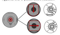
The valve shaft is at the position shown as on the left, the valve is closed, and the actuator pointer is at the "0" position.
