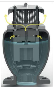
Air Release in Operational Conditions While in operation, the air generated by the pipeline accumulates in the upper section of the air valve. Gradually, it undergoes compression, and the pressure reaches the water pressure level. Consequently, its volume expands, pushing the water level downward and facilitating the release of air through the nozzle.
