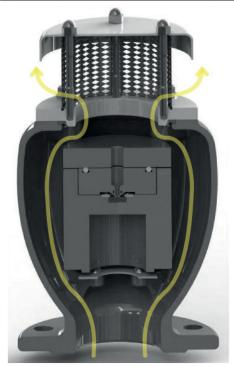
Discharge significant air volumes When filling the pipe, it's essential to release air while water enters. The A300X equipped with an aerodynamic full-port body and deflector, ensures the prevention of premature closures of the mobile block during this phase.
